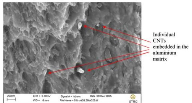
Fig. 6 Deformed and fractured particle of 2 wt.% CNT–Al (48 h MA), showing individual CNTs embedded in the aluminium matrix after the longest milling time of 48 h
