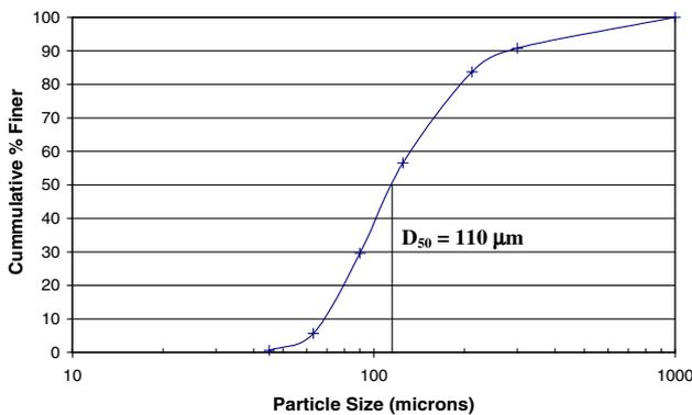
Fig. 4 Cumulative particle size distribution of 5 wt.% CNT–Al powders mechanically alloyed for 48 h
