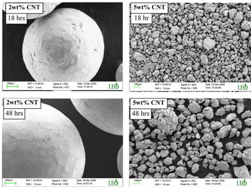
3 h. However, after 6 h, at which time smooth-surfaced large particles had been formed, no nanotubes were observed on the surface. It was assumed that by this stage the nanotubes were already embedded in between the welded particles. Deforming the large
