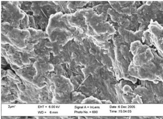
**Fig. 7** Particle of 5 wt.% CNT–Al (3 h MA), showing individual CNTs embedded in it
