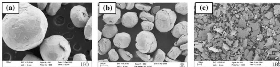
**Fig. 9** 2 wt.% CNT–Al after 12 h MA (a) with no PCA added, (b) with 0.1 wt.% PCA, (c) 0.7 wt.% PCA, showing flake morphology with addition of 0.7 wt.% PCA
