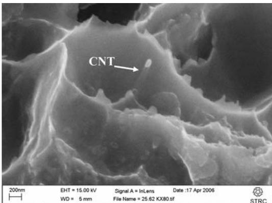
**Fig. 8** Deformed and fractured particle of 5 wt.% CNT–Al (48 h MA), showing a CNT embedded in the aluminum matrix
