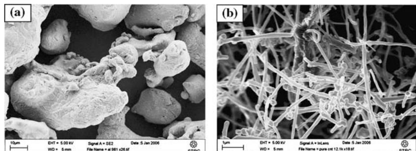
**Fig. 3** SEM micrographs showing particle morphology and size change with mechanically alloying time for 2 and 5 wt.% CNT–Al powder composites
