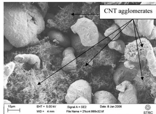
**Fig. 2** Clusters on nanotubes after dry mixing in a Turbula mixer
