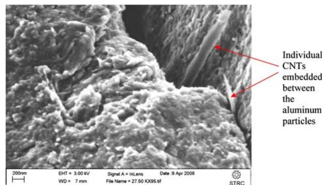
**Fig. 10** 2 wt.% CNT–Al (6 h MA with 0.1 wt.% PCA), showing individual CNTs being embedded between the aluminum particles
